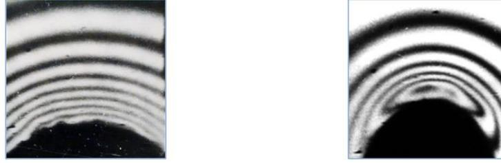
FIGURE 6 – Kerrograms — bands of equal phase shift  $\Delta\Phi$  between ordinary and extraordinary rays
