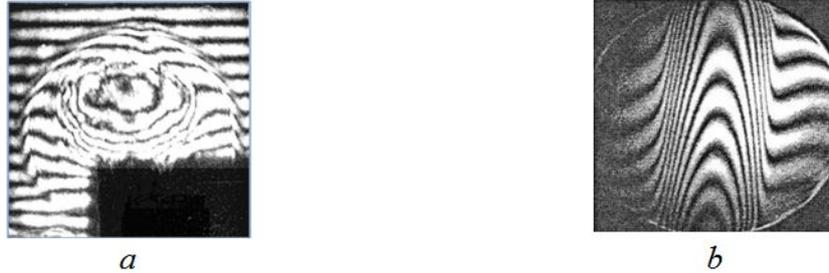
FIGURE 9 – Holographic and classical interferograms when tuned to finite width bands: a — holographic interferogram of a plasma bunch output from the electric breakdown channel of a solid dielectric [15]; b — classical candle flame interferogram [16]
