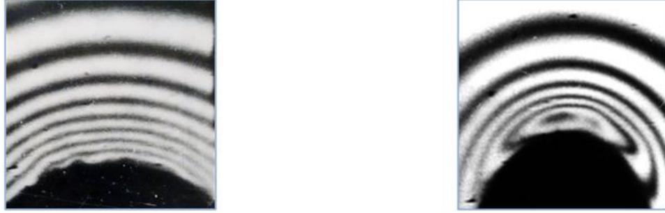
FIGURE 8 – Kerrograms — bands of equal phase shift  $\Delta\Phi$  between ordinary and extraordinary rays
