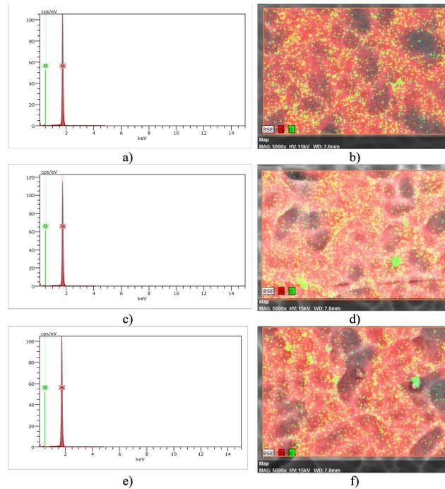
FIGURE 2 – EDX results of irradiated samples: a); c); e) EDX spectra for fluences  $3 \times 10^{15}$ ,  $1,15 \times 10^{16}$ ,  $1 \times 10^{17}$ , respectively; b); d); f) their corresponding element distribution maps
