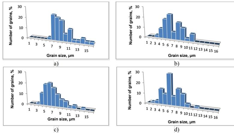
FIGURE 5 – Grain size distribution: a) initial b)  $3 \times 10^{15}$  ; c)  $1,15 \times 10^{16}$  ; d)  $1 \times 10^{17}$
