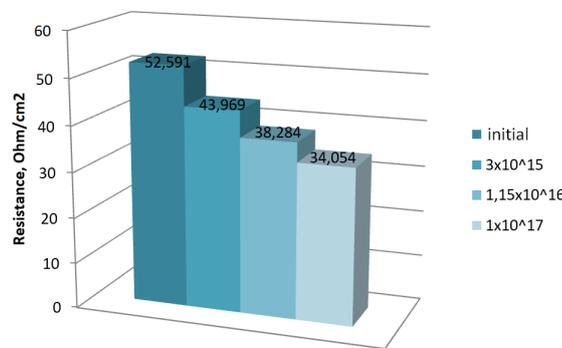
FIGURE 6 – Dependence of the change in electrical resistance on the irradiation fluence.
