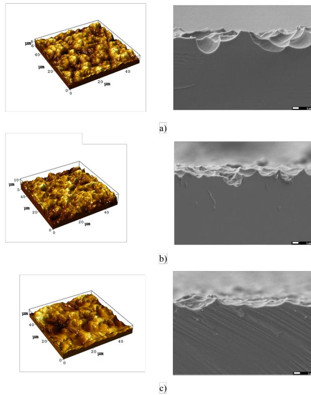
FIGURE 3 – AFM three-dimensional model of the surface and SEM image of the side cleavage of irradiated samples: a)  $3 \times 10^{15}$ , b)  $1,15 \times 10^{16}$ , c)  $1 \times 10^{17}$
