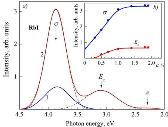
FIGURE 1 – *a*) The XRL spectra of a RbI crystal measured at 85 K without (curve 1) and under applied uniaxial elastic deformation with  $\varepsilon = 0.8-1.0\%$  (curve 2). Dashed lines demonstrate the spectrum decomposition into elementary Gaussians.
