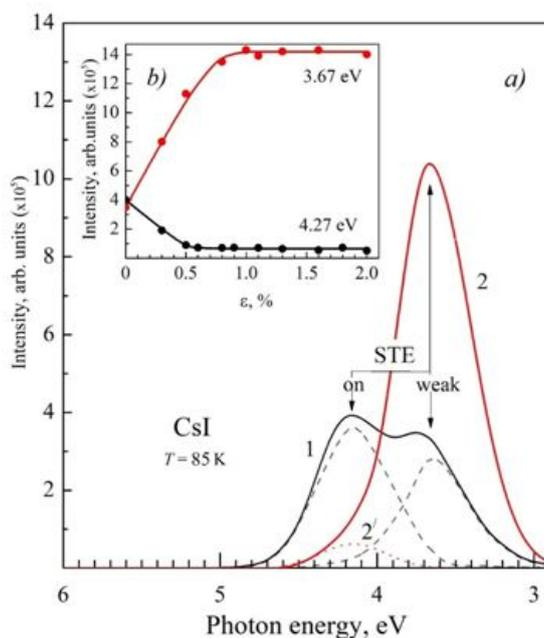
FIGURE 3 – a) The XRL spectra of a CsI crystal measured at 85 K without (curve 1) and under applied uniaxial elastic deformation with  $\varepsilon = 0.5\%$  (2). Dashed lines demonstrate the spectrum 1 decomposition into elementary Gaussians. Curve 2' - is a residual fraction of the spectrum 2 with respect to the  $\pi$  - STE Gaussian. b) The dependences of the intensity of the emission bands peaked at 3.67 eV (curve 1) and 4.27 eV (curve 2) on the degree of uniaxial deformation at 85 K.
