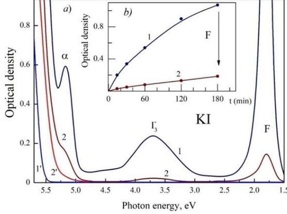
FIGURE 4 – a) The absorption spectra of a KI crystal measured at 85 K before (curves 1' and 2') and after isodose (3 hours) X - ray irradiation at 85 K (curves 1 and 2). The spectra correspond to an undeformed crystal (curves 1' and 1) and the sample exposed to a uniaxial stress with  $\varepsilon = 1.5\%$  at 85 K (curves 2' and 2).
