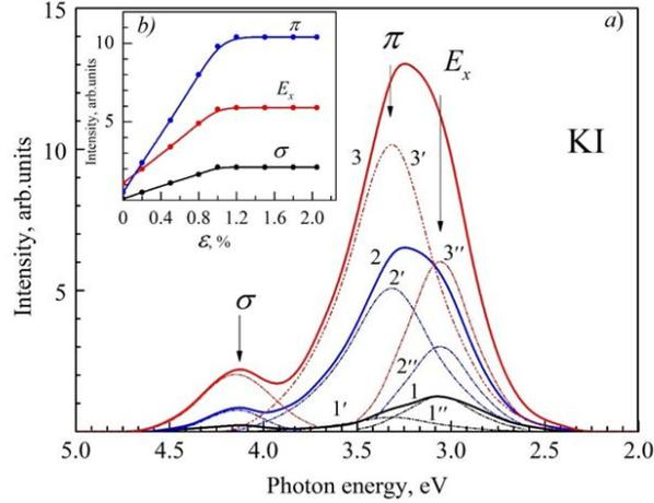
FIGURE 2 – *a*) The XRL spectra of a KI crystal measured at 85 K without (curve 1) and under applied elastic uniaxial deformation with  $\varepsilon = 0.5\%$  (curve 2) and  $\varepsilon = 1\%$  (curve 3). Dashed lines demonstrate the spectra decomposition into elementary Gaussians.
