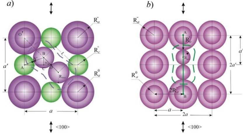
FIGURE 5 – A stoichiometric model describing the stabilization of an H center in *bcc* (a) and *fcc* (b) AHC lattice.
